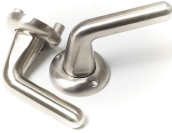
34813 Anti-ligature short lever set Solid Stainless steel 50mm rose Heso type spindle heavy duty bolt through fixings 8mm spindle for doors 44mm-60mm
